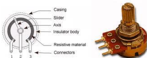
Figure 2: Potentiometer
